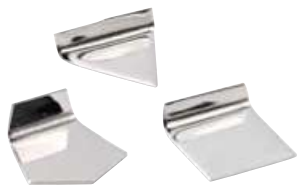
Milligram weights, flat polygonal sheet
