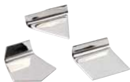
Milligram weights, flat polygonal sheet
